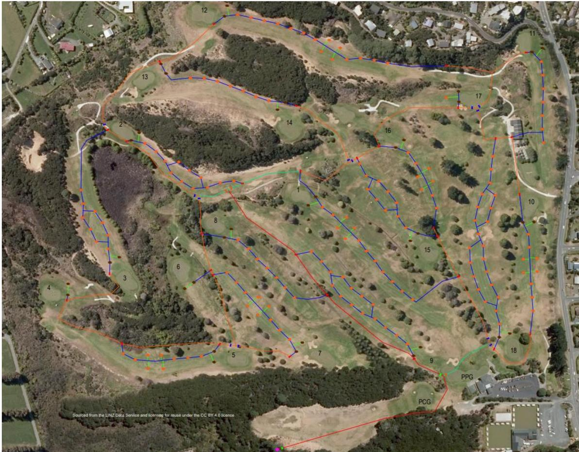
Figure 5-2 Proposed Wastewater Irrigation System
